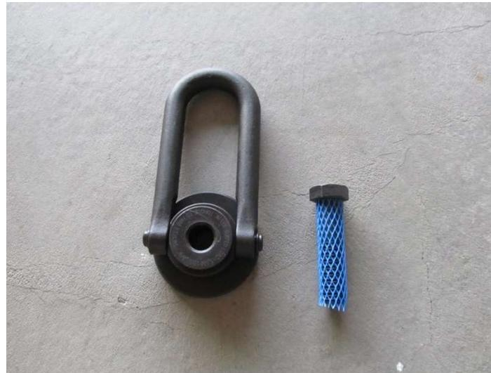
THE SINGLE RIGGING PICK POINTS FOR STEEL ARE EASILY INSTALLED ON ANY STEEL STRUCTURE WITH ANY LENGTH OF BOLT OR THREADED ROD. THEY HAVE A WLL OF 2,500 LBS OR 5,000 LBS IN ANY DIRECTION. THIS LIFTING DESIGN COMES AS A KIT WITH EVERYTHING YOU NEED TO QUICKLY INSTALL A SINGLE RIGGING PICK POINT ON YOUR STEEL STRUCTURE. ALSO OSHA APPROVED FOR FALL PROTECTION.
